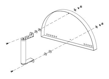
6/. Installed chimney cap with 4pcs of 5/32"\*10mm screws
