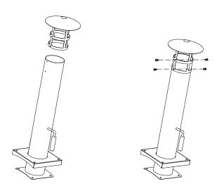
7/. Installed Chimney with 4pcs of 1/4"\*15mm screws
