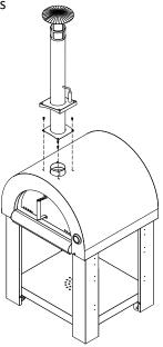
8/. Installed chimney box with 4pcs of 1/4" 30mm screws
