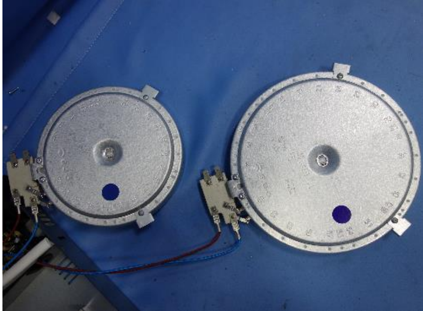
View of Heater Element
