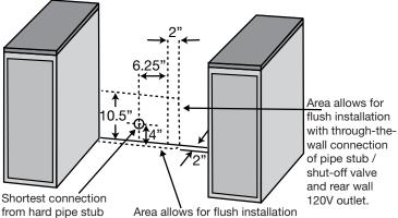
with through-the-floor connection location to range of pipe stub / shut-off valve.
